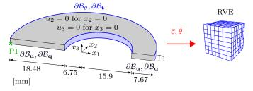
water cooling is applied on the lateral surface as Dirichlet bc's
